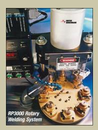
Pre- and post-weld station part sensors and head retract sensor verify part presence and head position, inhibiting rotation and welding if error condition exists. If pre-weld station senses missing part, that position will be skipped.
