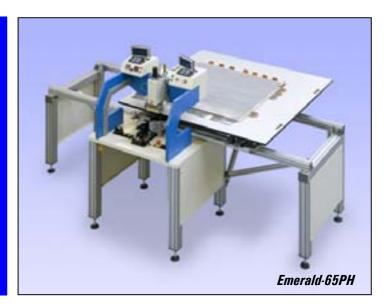
UNITEK EAPRO offers a full product line of LCD/PDP Bonding and Repair systems. The Emerald Series are designed for a wide variety TAB/COG/Flex sizes and can handle panel sizes ranging from 1" up to 65". The Emerald highly flexible system can be used for ACF Tacking, ACF Final Bonding and Hot Bar Soldering.
