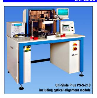
The Uni-Slide/Uni-Slide Plus Systems have a product handling slide in the front-rear direction. The slide system moves the products from the operator position to the processing position. In the processing position the bonding head moves the Thermo-Plane Thermode on top of the products to be bonded.
