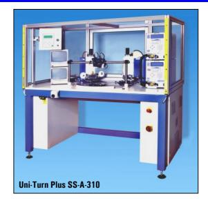
The Uni-Turn/Uni-Turn Plus Systems use a rotary table that rotates the products from the operator position to the processing position. These Systems offer maximum output due to the simultaneous loading/unloading and bonding of the product. The loading position is always located in front of the operator making these systems ergonomically friendly. Both Systems can use either the SH500 (pneumatic) or PH500 (motorized) bonding heads.
