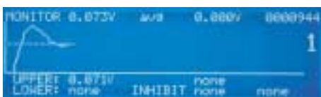
Monitor Screen – Shows 1st Pulse weld current exceeded limit.
