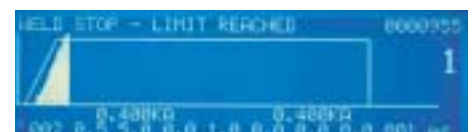
Run Screen – Shows termination of weld current during weld pulse.
