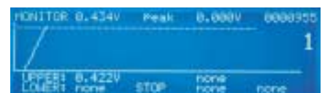
Monitor Screen – Shows weld current exceeding limit.
